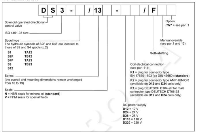
This version enables hydraulic actuators to perform a smooth start and stop by reducing the speed of movement of the valve spool.
