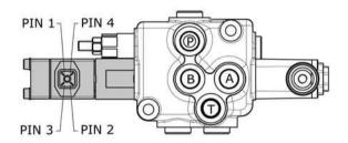
**CONTROL in A e B** = connect PIN 1 - 4 and 2 - 3 **CONTROL in A** = connect PIN2 - 3
