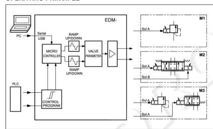
The EDM-M\* card is a digital amplifier for open loop proportional valves control by a PWM stage.
