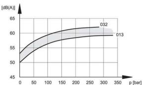
The noise pressure levels were measured in a semianecoic room, at an axial distance of 1 m from the pump.
