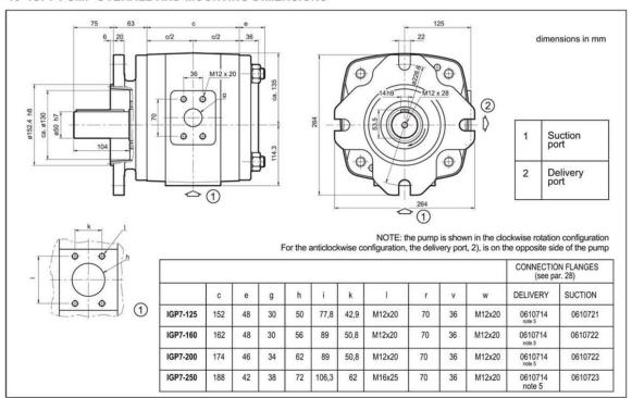
NOTE 5: For applications with delivery pressure greater than 200 bar, it is necessary to use the special connection flange, code 0610725.
