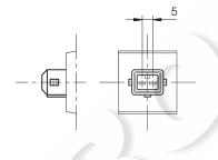
connection for DEUTSCH DT06-2S male connector type code **K7**
