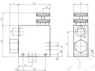
These flow regulators are pressure compensated and limit the outlet flow from the regulated "R" port at a constant adjustable level. largely independent from load and pressure changes.
